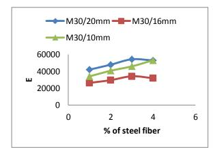
Fig 9:EVs% of steel fiberforM30
